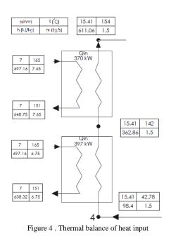
Heat input section contain 2 heat exchanger, preheater and evaporator. The preheater raised the temperature to the saturation liquid point, before it continued to the evaporator, which boiled the water to the saturation vapor point. As shown in Figure 4 is the parameters output for this section.
