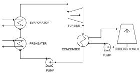
Figure 3 ORC Schematic Diagram
