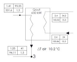
Figure 5. Thermal balance of condencer
