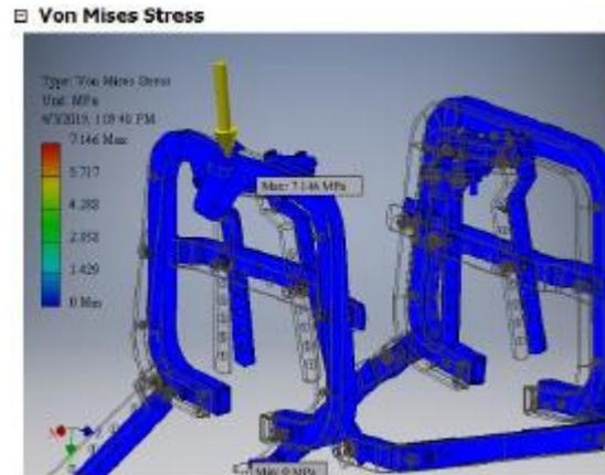
Gambar 8 Simulasi Von Mises Stress
