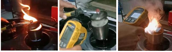
Gambar 11. Proses uji temperatur autoignition
