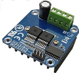
**Gambar 5.** Motor Driver BTS7960 43A
