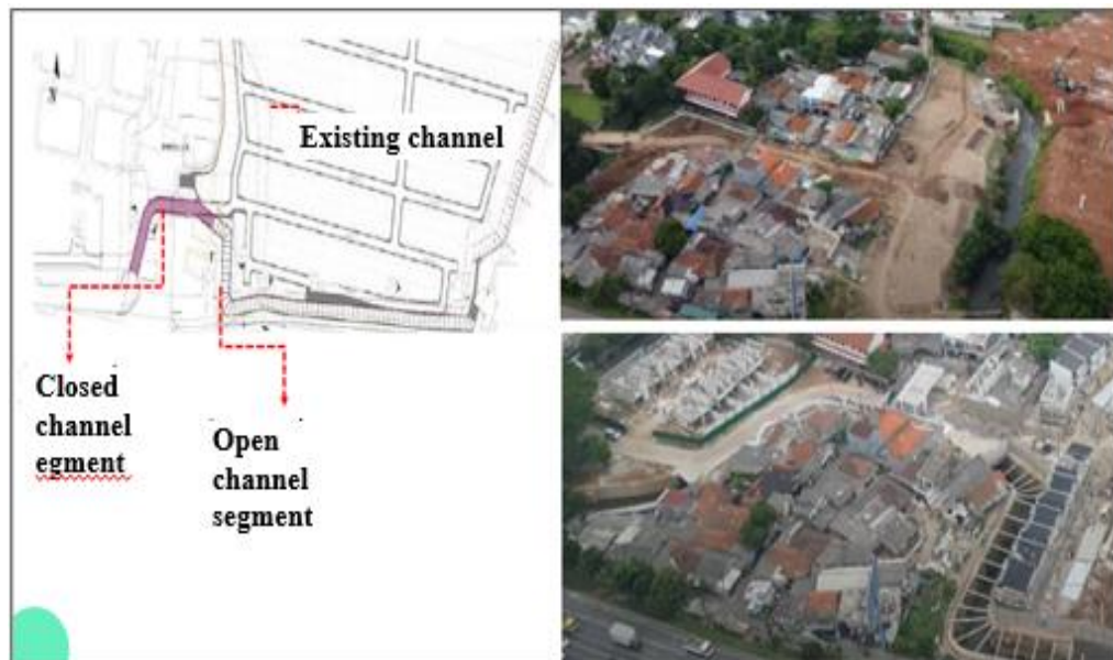
Figure 6. Overview of the Channel Diversion Project. Source: Project Processed Data 2023
