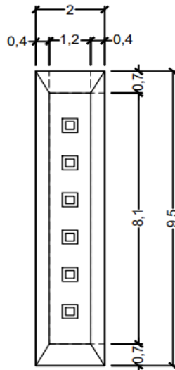
Figure 10. Abutment 2 Redesign Top View
