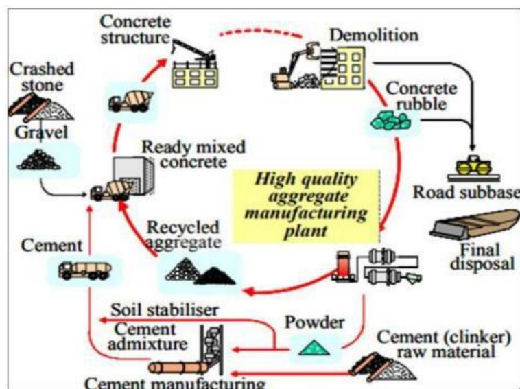
Figure 2. Schematic flow of concrete recycling system
