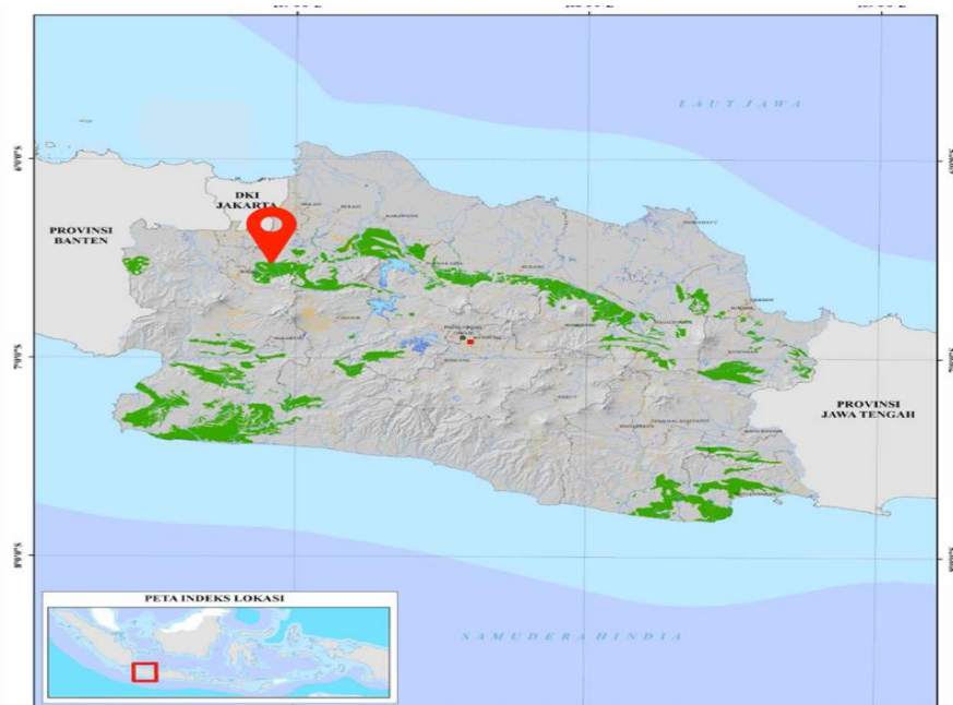
Figure 1. The map of the spread of problematic clay in west java [8]
