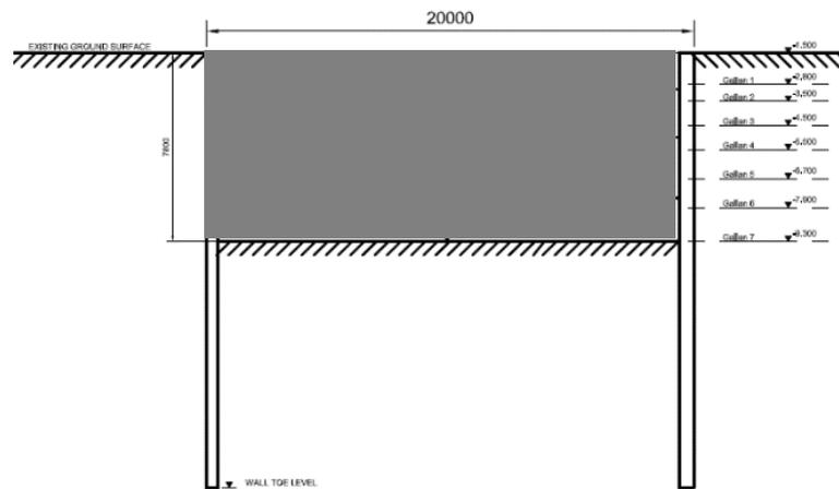
**Figure 4.** Excavation plan phase 1
