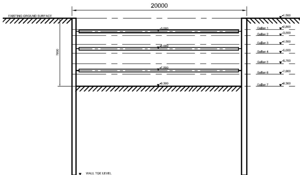
**Figure 3.** Sections of the foundation excavation plan
