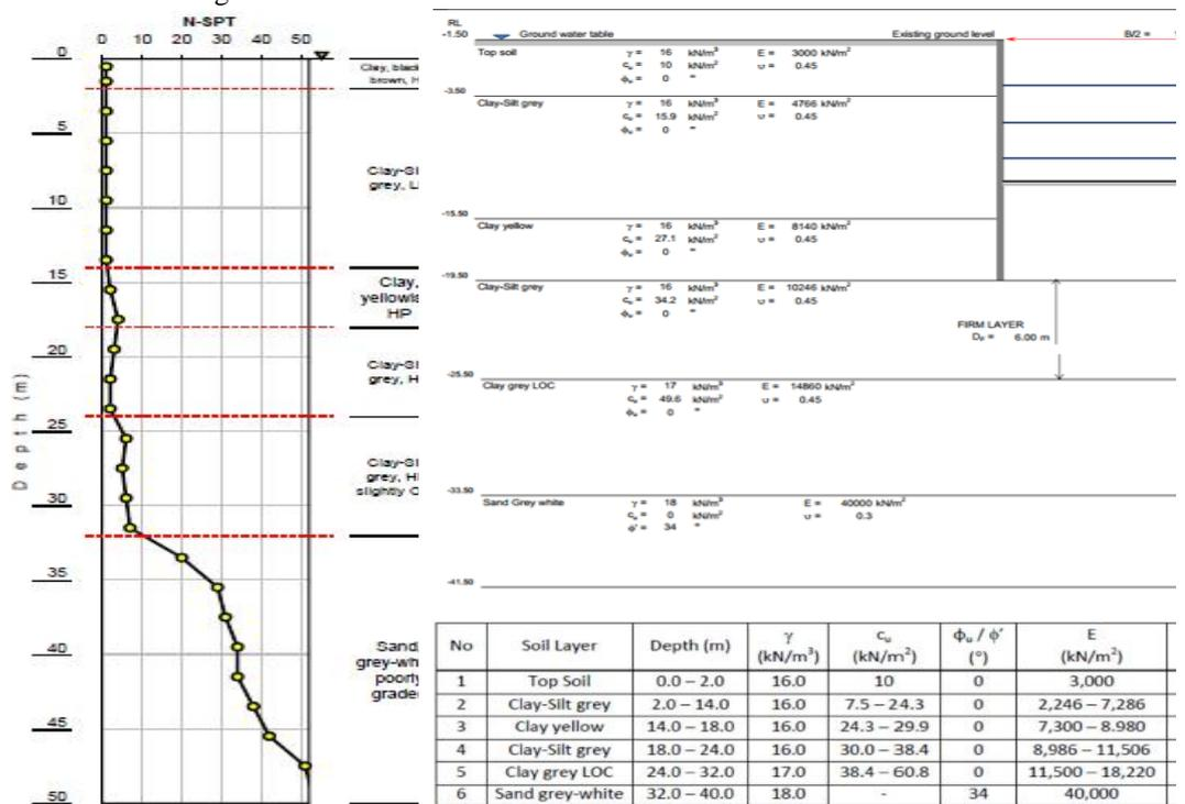
**Figure 1.** Soil profile and interpretation of soil data Source: Lab Documentation. Soil Mechanics, 2019.
