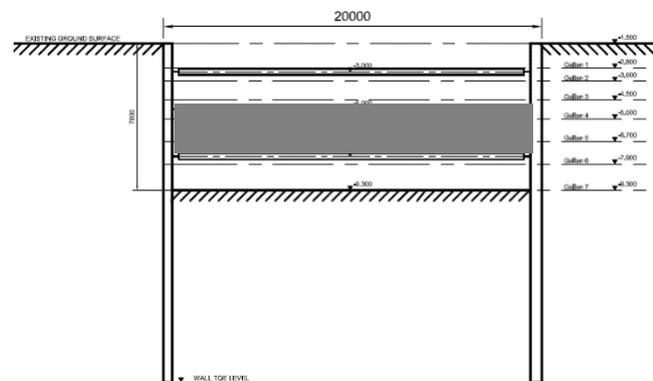
**Figure 8.** Excavation plan phase 5
