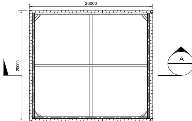
**Figure 2.** Top view of the foundation excavation plan
