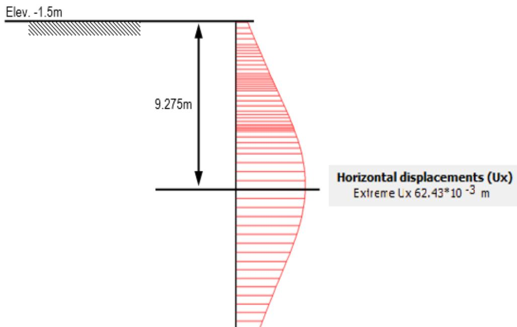
**Figure 13.** Lateral movement occurring at the end of construction
