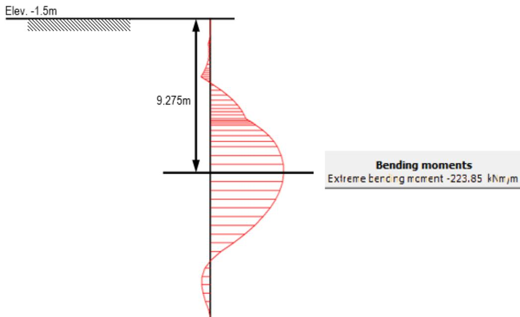
**Figure 12.** Maximum moment that occurs in the sheet pile system
