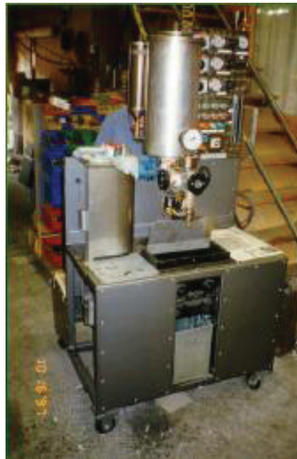
Figure 2. Wirtgen WLB 10 Equipment
