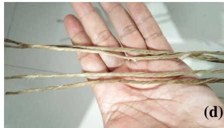
Figure 2. Process of water hyacinth fiber treatment: (a) shredded water hyacinth, (b) soaking with NaOH, (c) drying again, (d) rolling water hyacinth fiber
