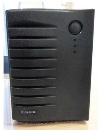
Gambar 18 Uninterruptible Power Supply
