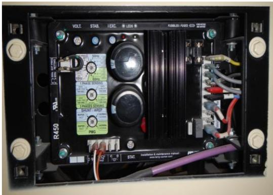
Gambar 2. Automatic Voltage Regulator (AVR)
