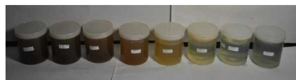
Figure 11. Samples of flotation with 15 V voltage, liquid plus ethanol
