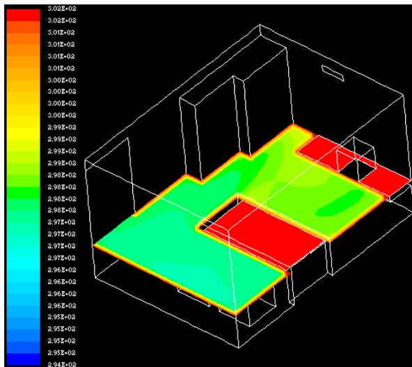
Figure 15. Full temperature contour around meeting area of case 4
