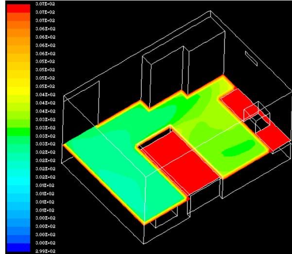
**Figure 9.** Full temperature contour around meeting area of case 1
