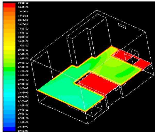
**Figure 13.** Full temperature contour around meeting area of case 3
