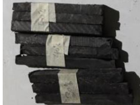
Gambar 3.5 specimen uji impact
