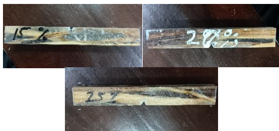
Gambar 3. Sampel Uji Impact
