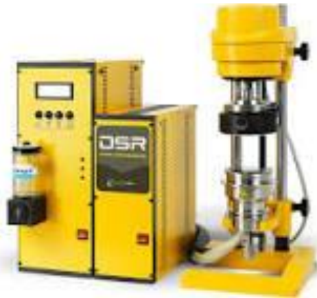
Gambar 9. Alat Dynamic Shear Rheometer
