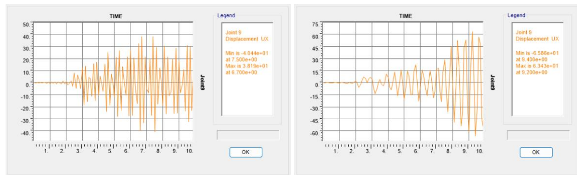
(a). RISHA type 36 without isolator. (b). RISHA type 36 with isolator. Figure 13. Lateral eformation lateral due to Pacoima Dam earthquake load (unit: mm).
