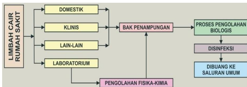
Gambar 4 Diagram pengolahan air limbah
